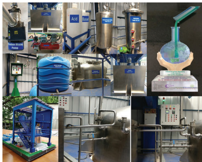
Fig. 12: A 10 m 3 pilot plant for the production of biohydrogen from waste installed and operated at CSIR-IICT
