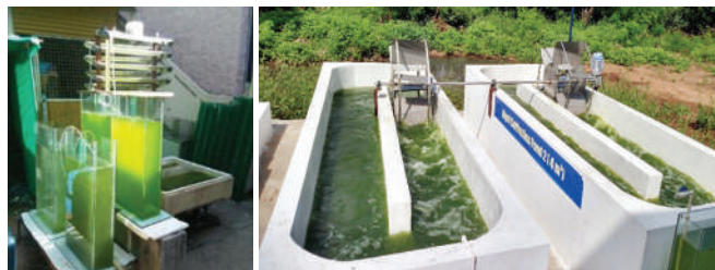
Fig. 9: Flat Panel and Raceway pond (3000 liters) systems for algal cultivation designed and developed at CSIR-IICT
