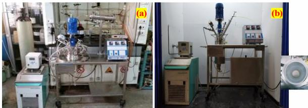
Experimental setup(a) 1L SS Reactor, and (b) 2L PTFE lined SS Reactor
