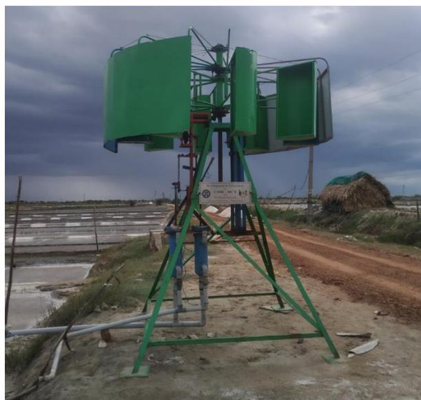
Mastless windmill designed, fabricated at CSIR-ICT and installed at West Gogulapalli
