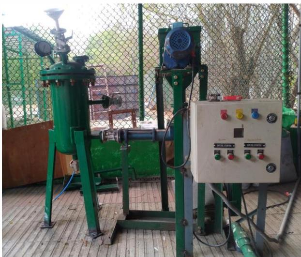
Reactor operated with Lignocellulosic biomass
