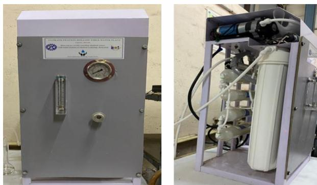
Mini pilot plant of 100 LPH capacity with frontal, and lateral view
