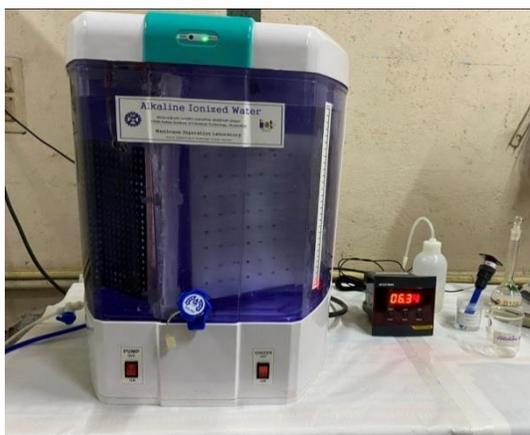
Alkaline Ionized Water Electrolyzer
