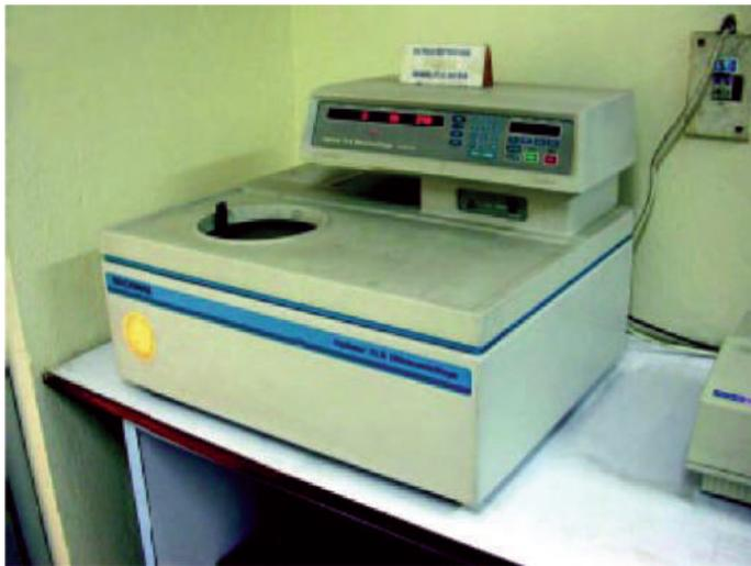
The Beckman Coulter Optima TLX Ultracentrifuge is a tabletop ultracentrifuge that can be used for many types of high-speed applications. Some of the features of the Optima TLX include an easy to use control panel, a temperature control system, a self-purging vacuum system, a programmable memory that can store up to 10 different profiles and a versatile acceleration/deceleration program. In addition, because this instrument has a maximum speed of 120,000 rpm, it comes with many safety features.
