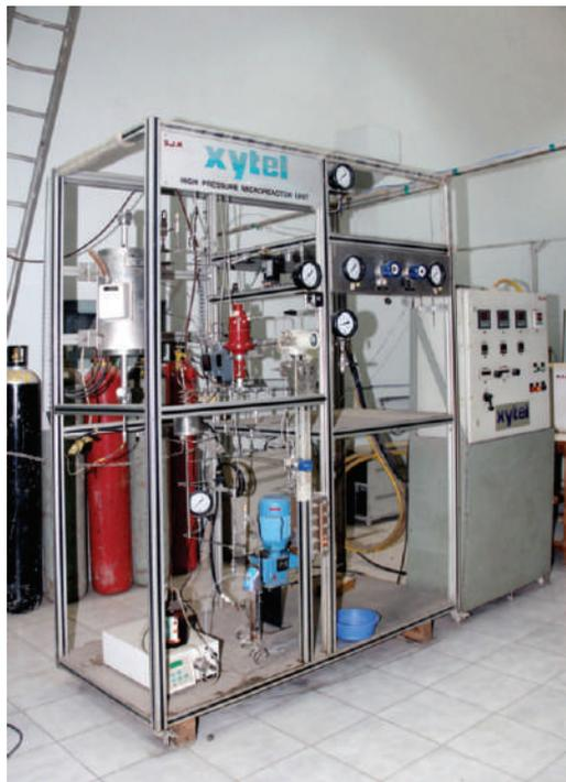
High Temperature single tube Catalytic fixed-bed reactors are the most important type of reactor for the synthesis of basic chemicals and intermediates. In these reactors, the reaction takes place in the form of a heterogeneously catalyzed gas reaction on the surface of catalysts. In addition to the synthesis of valuable chemicals, fixed-bed reactors have been increasingly used in recent years to treat harmful and toxic substances.
